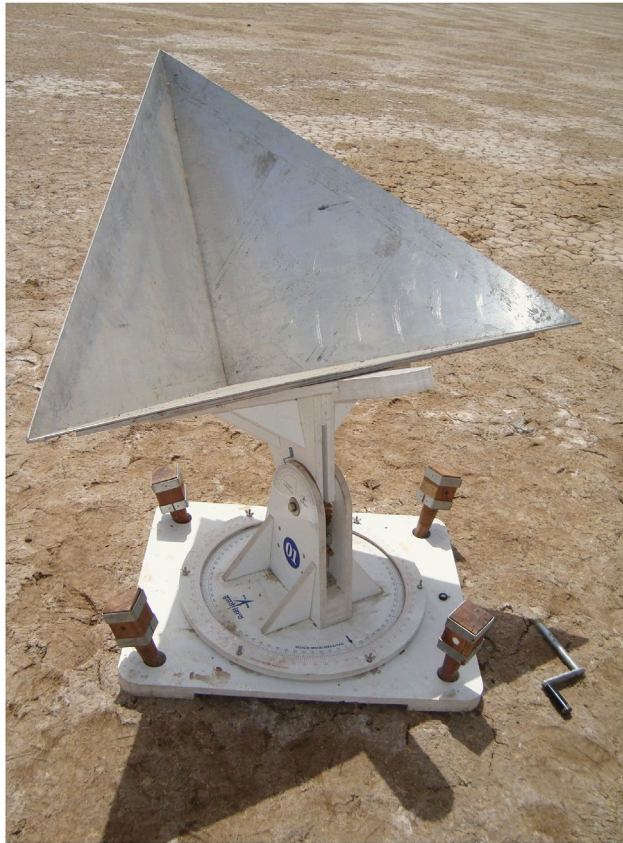
Figure 2. Corner reflector at calibration site, Desalpar, Rann of Kutch.
