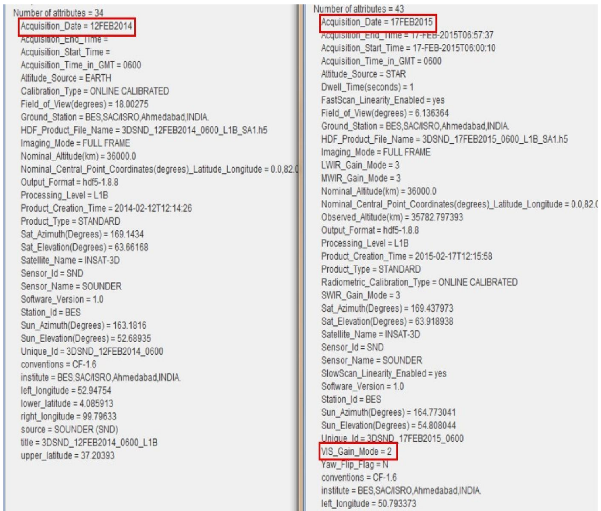
Figure 15: The change in gain mode for visible channel of INSAT-3D sounder.
