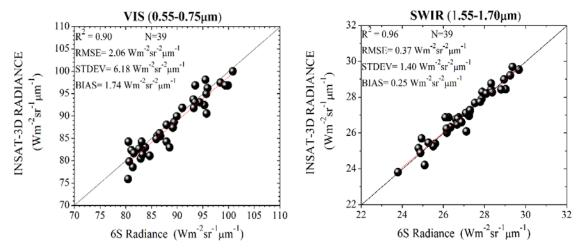
Figure 13: The combine linear regression between INSAT-3D measured and 6S simulated Radiance over GROK for Visible & SWIR channel for Year 2015
