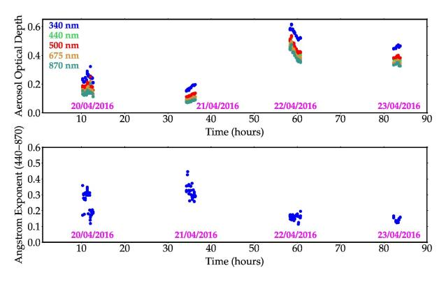
*Figure 8:* Upper panel shows the variation of aerosol optical depth at five different wavelengths (340, 440, 500, 675 and 870 nm) and lower panel shows the variation in estimated Angstrom Exponent at 440-870 nm
