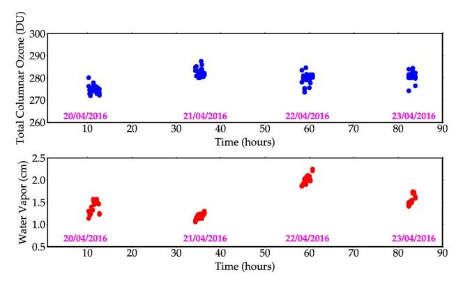
**Figure 9:** Upper panel shows the variation of Total columnar ozone in Dobson units and lower panel shows the variation of water vapour in cm measured using MicroTops-II ozonemonitor for all four clear-sky days
