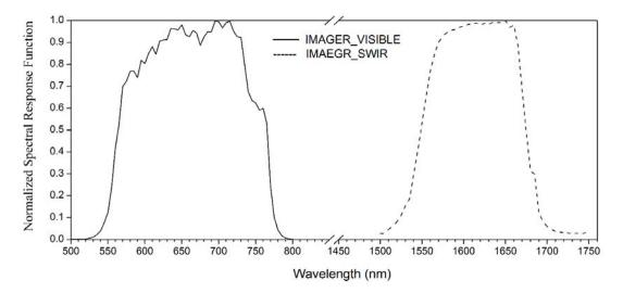
Figure 11: Pre-launch laboratory measurements of spectral response function for VIS and SWIR channels of INSAT-3D
