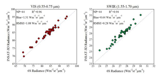
Figure 12: The combine linear regression between INSAT-3D measured and 6S simulated Radiance over GROK for Visible & SWIR channel for Year 2016
