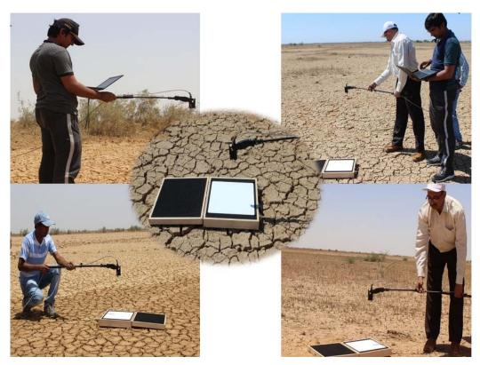
Figure 4: Collection of surface reflectance using ASD hyper-spectral radiometer during the campaign
