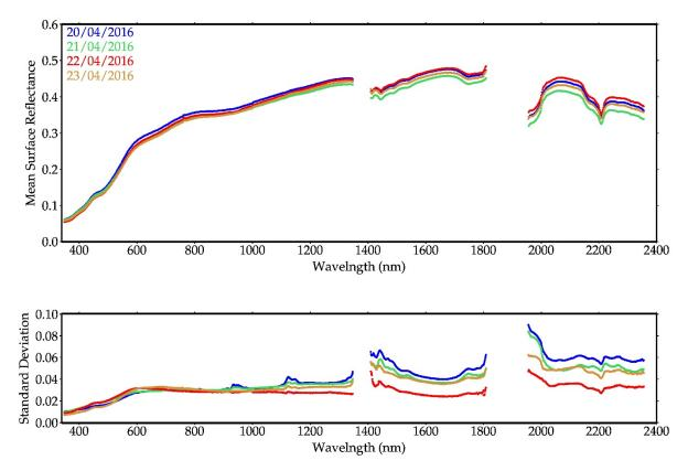
*Figure 6:* Daily averaged measured surface reflectance at GROK site for all four clear-sky days in upper panel and Lower panel shows the standard deviation in the measured surface reflectance
