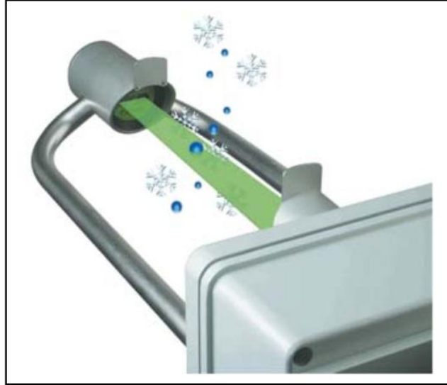
Figure 2: The working principle of OTT parsivel optical disdrometer Parsivel. The signal gets attenuated when pass through the signal (Courtesy: Thies Clima, 2007)
