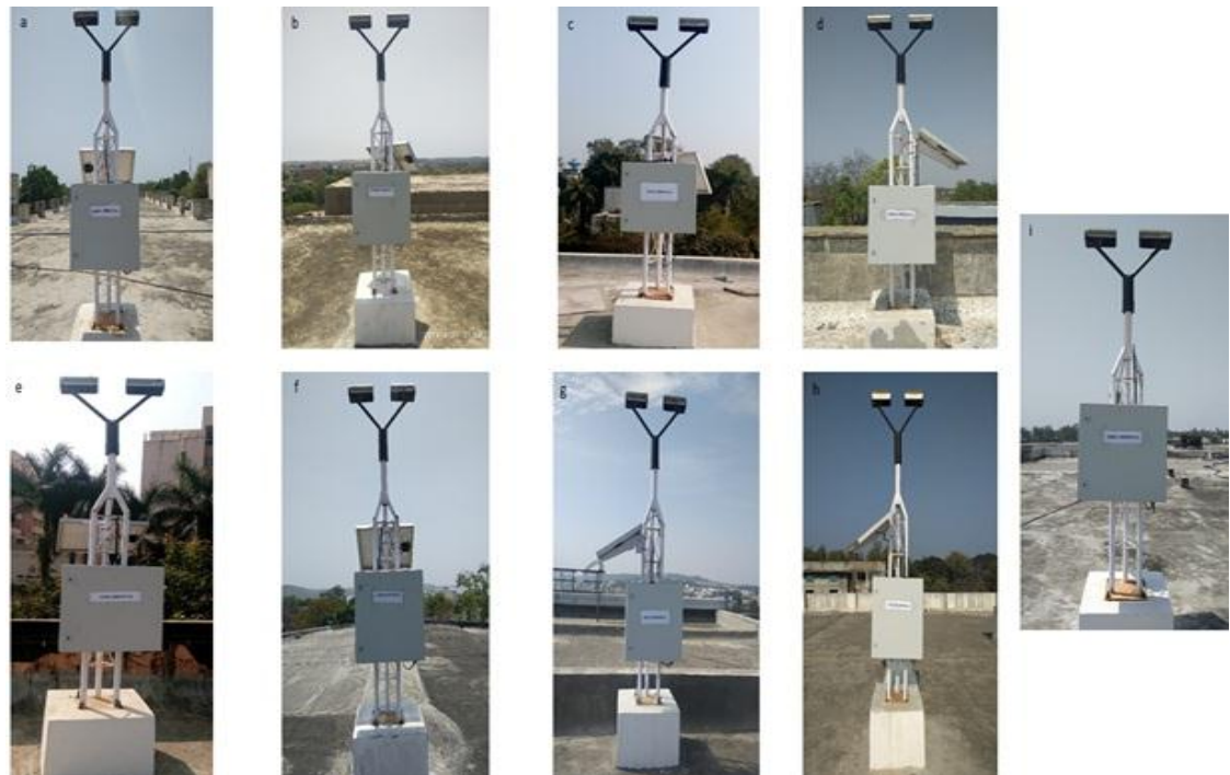
Figure 1: (A)The site locations and the (B)images of nine optical disdrometers installed over the site (a) BHEL (b) BMHRC (c) BSSS (d) IIFM (e) IMD (f) JDA (g) MPCST (h) NITTR (i) SIRT
