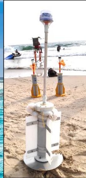
GNSS/NavIC drifter designed @SAC
