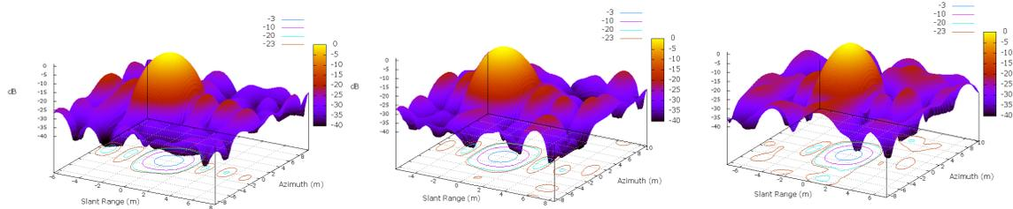
**Fig. 4:** Point target Impulse response Function for CH polarisation for point target 1, 2 and 3 (01Oct2013)
