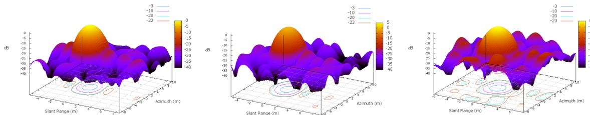
**Fig. 5:** Point target Impulse response Function for CV polarisation for point target 1, 2 and 3 (01Oct2013)
