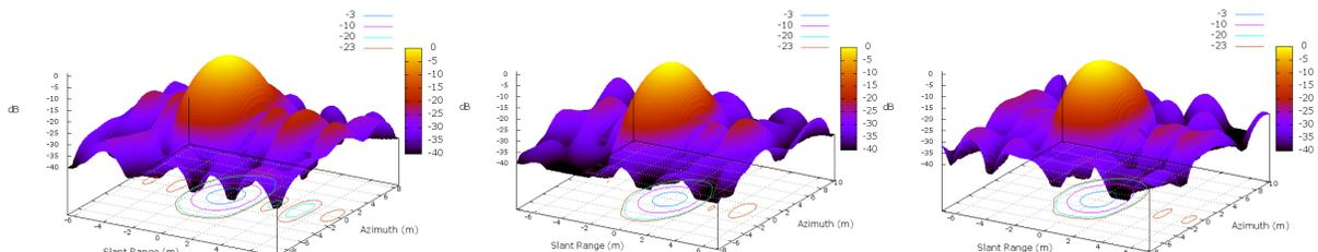
**Fig. 7:** Point target Impulse response Function for VV polarisation for point target 1, 2, 3 and 4 (02Jun2013)
