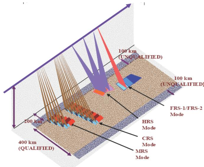
**Fig.1:** Schematic Diagram showing different beam modes of RISAT-1 SAR
