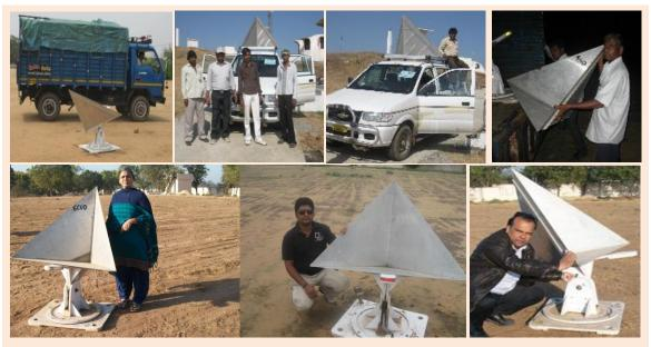
Fig.2: Corner reflector mobilization & deployment
