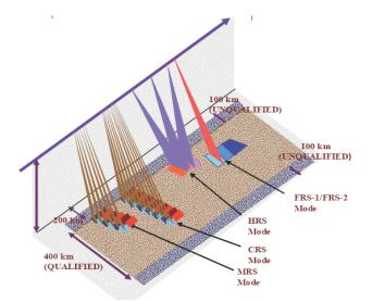
Fig.1: Schematic Diagram showing different beam modes of RISAT SAR
