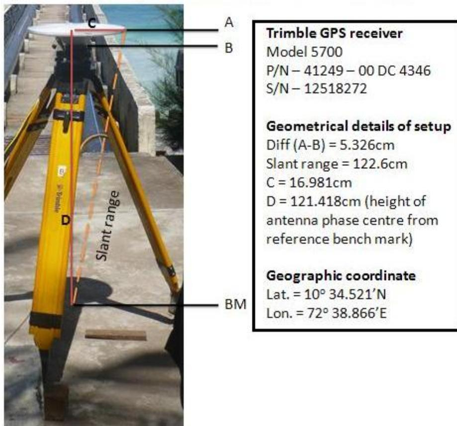
Figure 12b: GPS reference station at TG2 during levelling experiment
