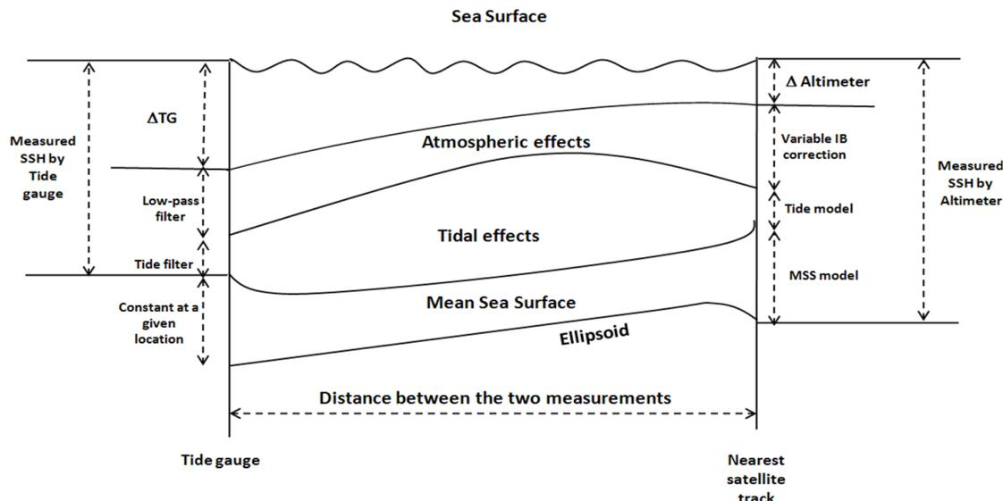
**Figure 19:** Schematic diagram of performing altimeter absolute calibration
