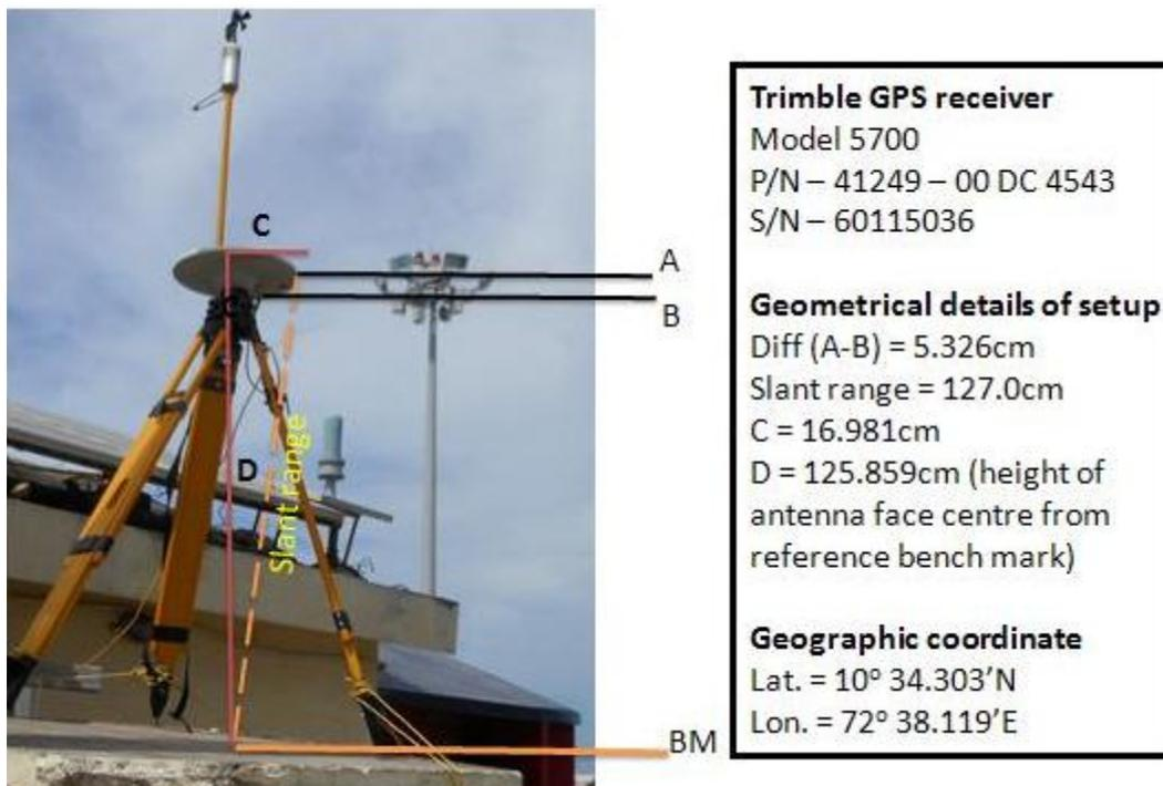
Figure 12a: GPS reference station at TG1 during levelling experiment
