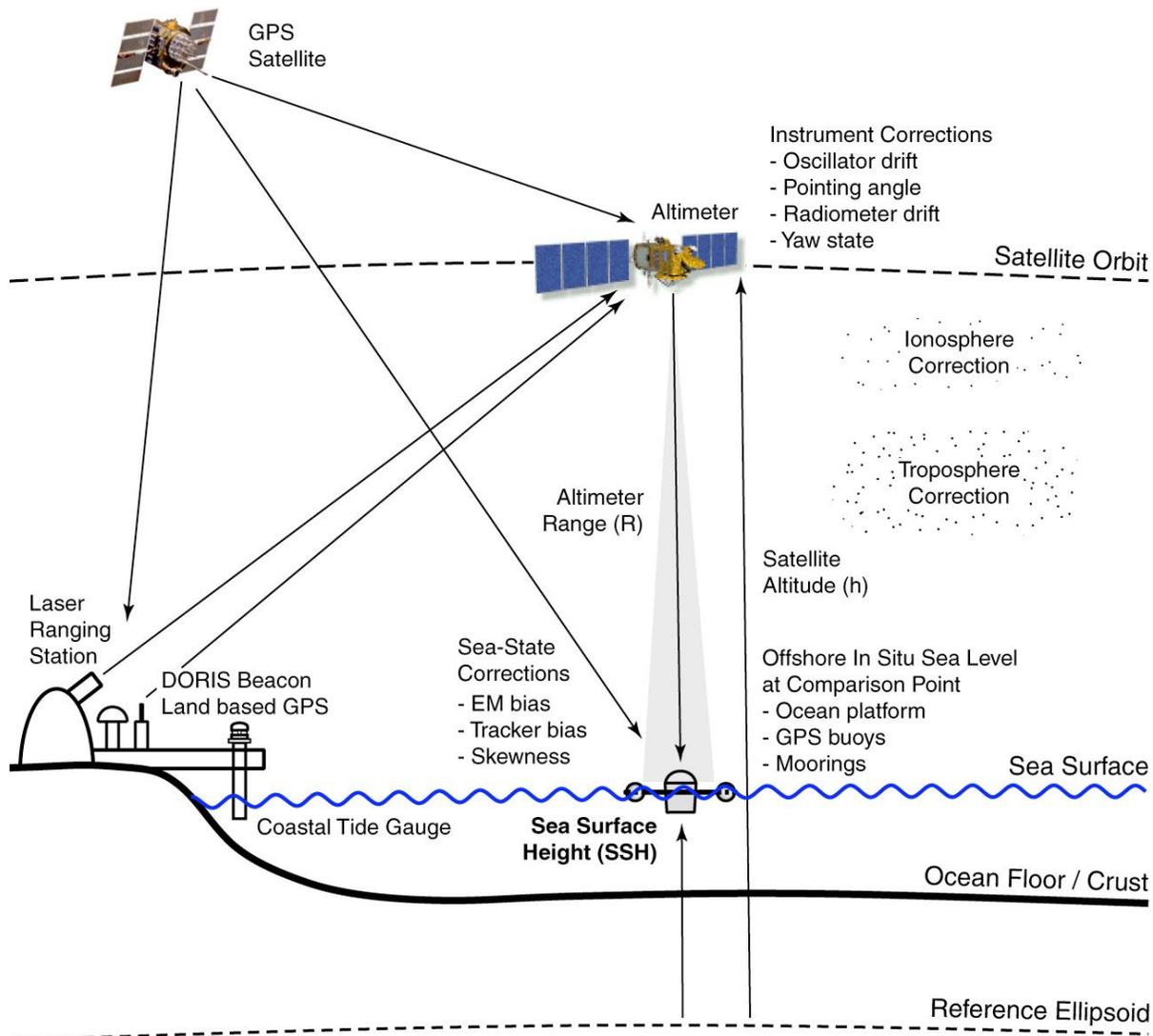
**Figure 18:** The schematic diagram shows altimeter point calibration geometry.
