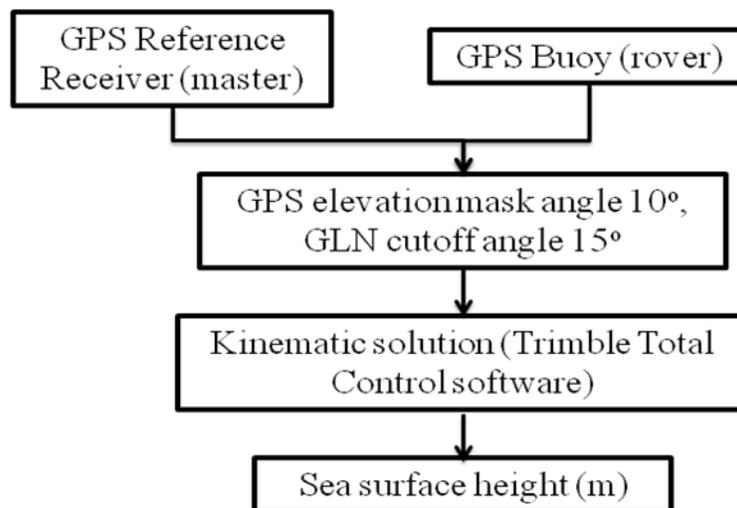
**Figure 14:** Flow diagram on derivation of SSH from GPS buoy.
