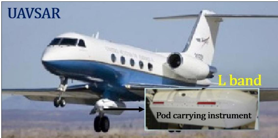
Figure 2. UAVSAR/Gulfstream-III at an airport. UAVSAR Antenna is contained in the pod mounted under the GIII body
