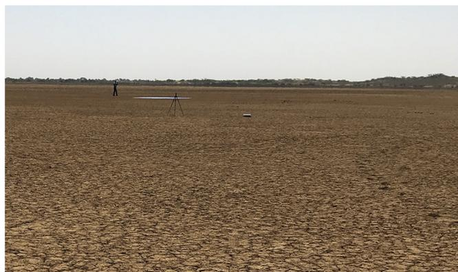
**Fig. 6.** Desalpar Playa, Gujarat Province, India. A spectralon panel, leveling tripod, and a tarp target used for localization are visible in the background.
