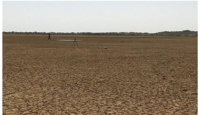
**Fig. 6.** Desalpar Playa, Gujarat Province, India. A spectralon panel, leveling tripod, and a tarp target used for localization are visible in the background.
