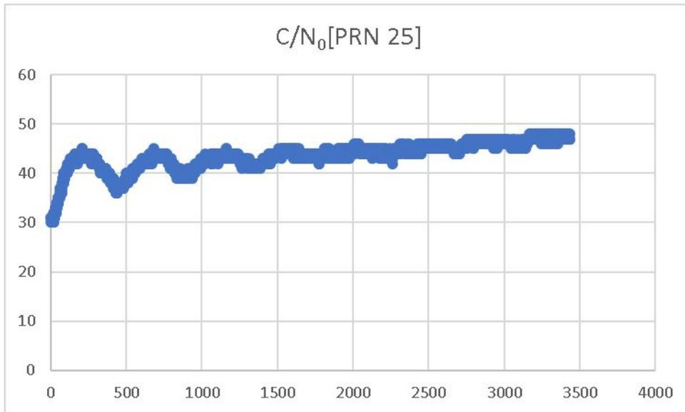
Figure 21: Interference pattern in C/N0 (SNR/BW) for satellite of PRN No 25
