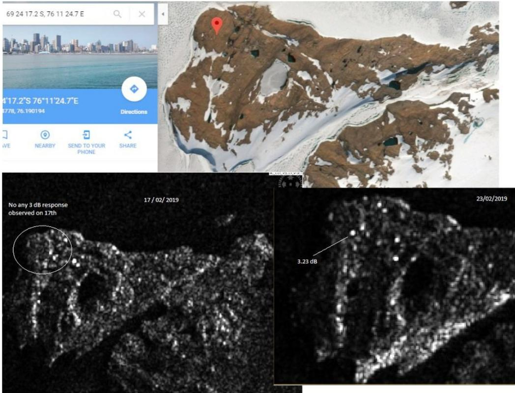
Figure 17: CR response deployed at Bharati in the image
