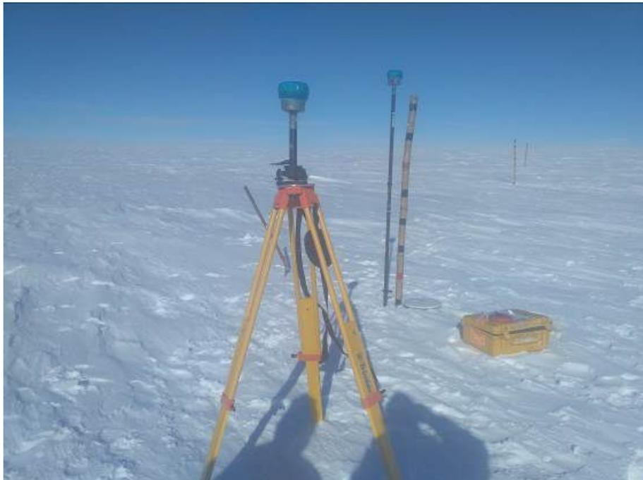
*Figure 11: DGPS measurement of newly installed Bamboo Stack at Polar Record Glacier.*
