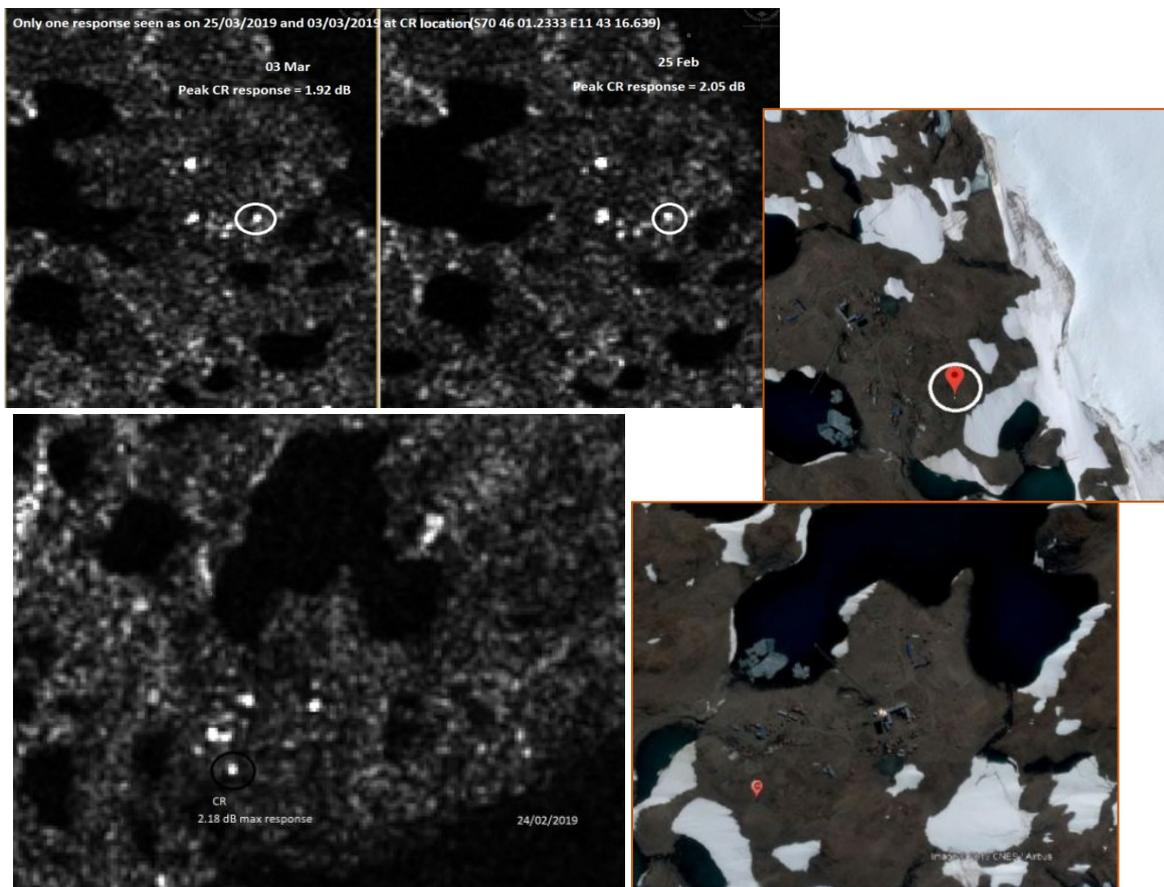
Figure 18: Response of Corner Reflector in the image on 24th Feb, 25th Feb and 3rd March at Maitri
