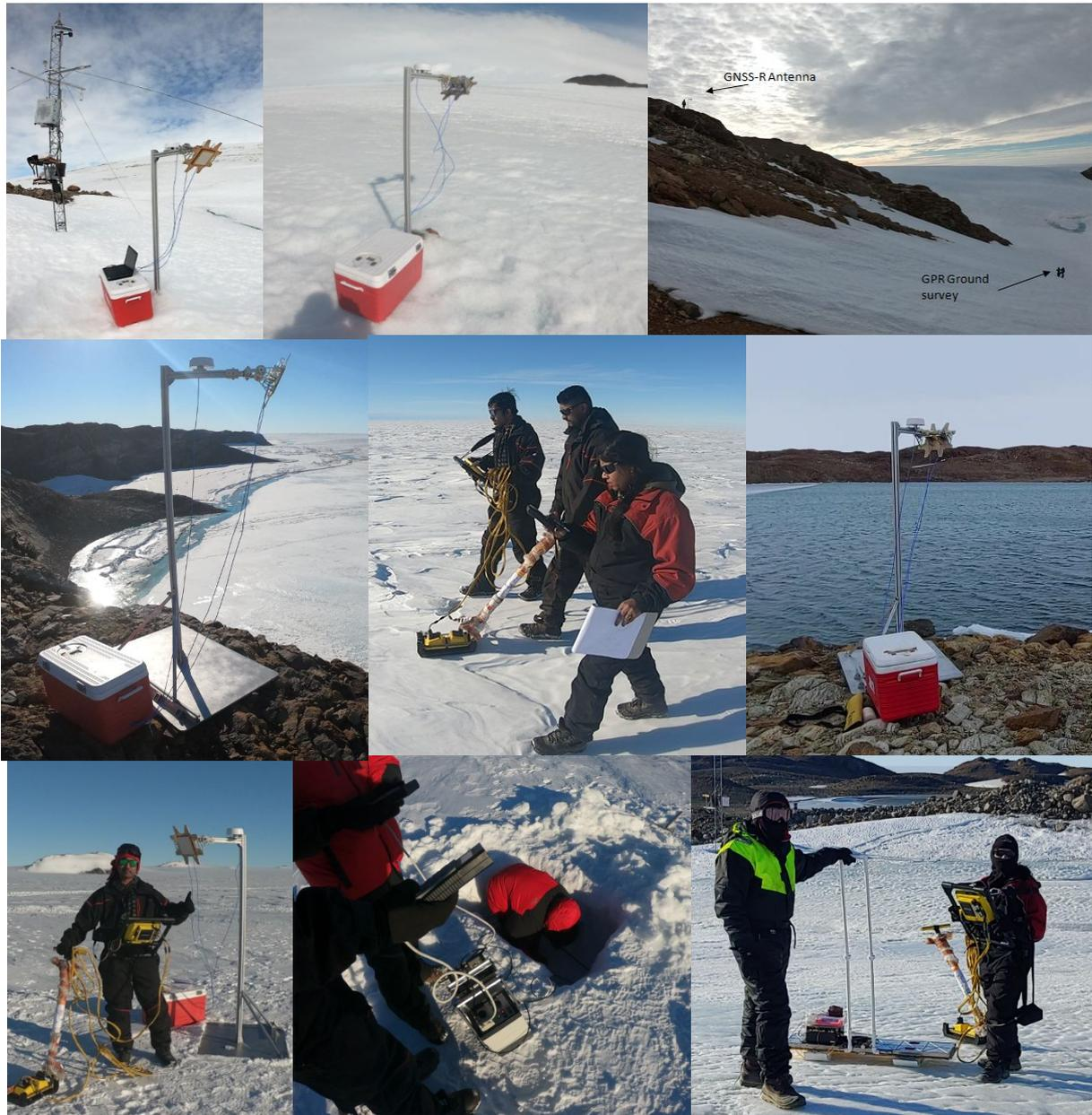
*Figure 8: GNSS reflectometry set-up*
