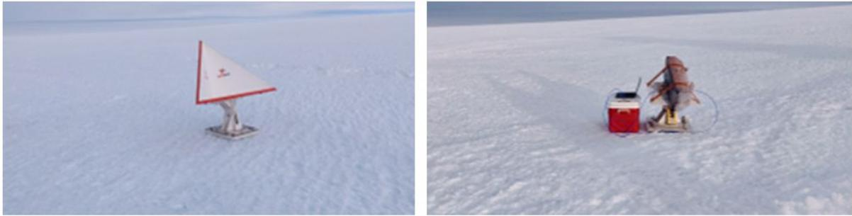
Figure 3: Deployed Corner Reflector and ARC at ice sheet on 8<sup>th</sup> Jan 2019
