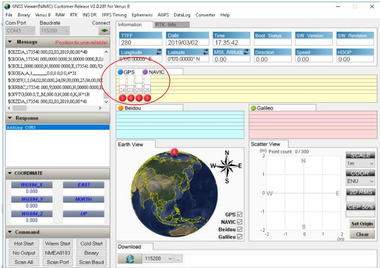
Figure 23: Detection of NavIC Signals at Maitri Antarctica
