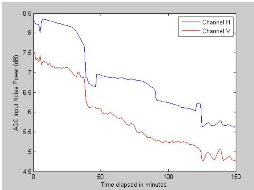
Figure 20: Output noise power of GNSS-R receivers' ADCs
