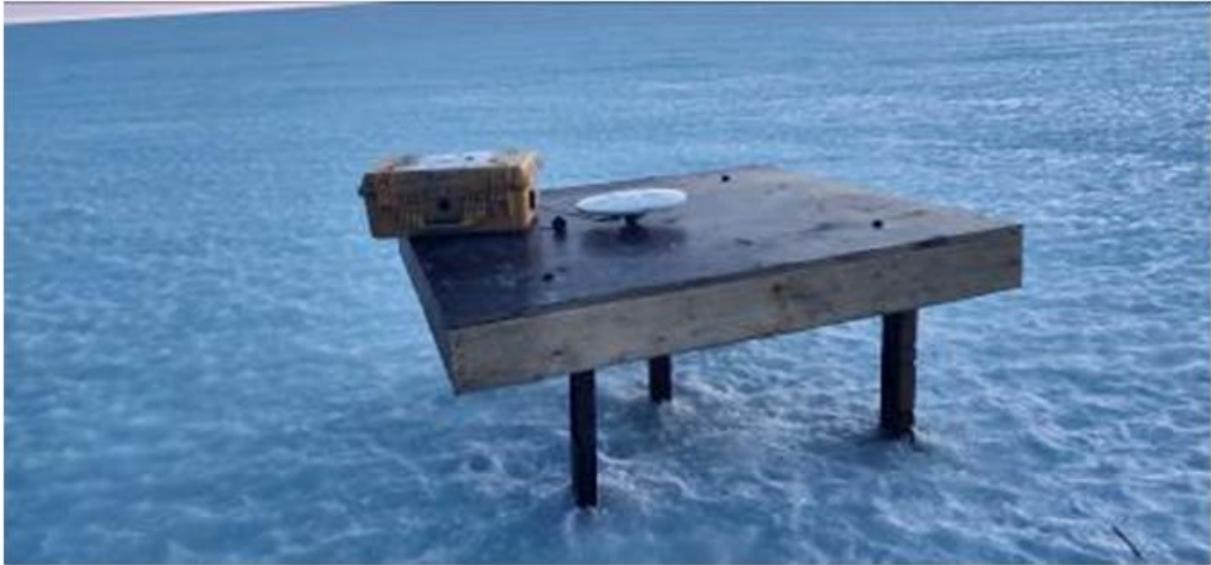
Figure 5: Installed wooden plank with ongoing DGPS measurements at Maitri
