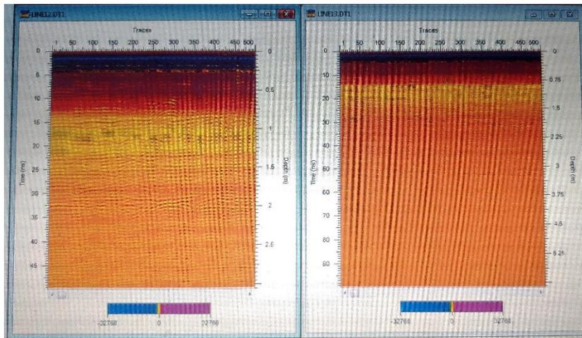
Figure 22: 1GHZ GPR data of 100ns (left) and 50 ns(right) time window for the same line
