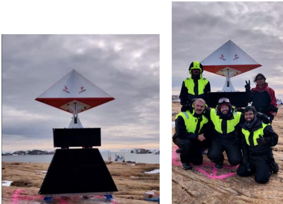
*Figure 7: Permanently Deployed Corner Reflector set-up at Bharati and the supporting team members*
